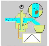
restricted flow path). The cloud of positive counter ions surrounding the colloid is stripped off resulting in a current flowing in the sensor. This is detected and output back to the controller.
